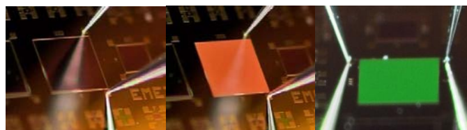
Figure 7. Pictures of the unbiased silicon nanocrystals (Si-NC) LED, an orange emitting Si-nc LED under forward bias and green emitting Si-nc:Er LED (from left to right).
